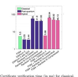
Certificate verification time (in ms) for classical, post-Quantum, and hybrid algorithms, achieving Security Level 3 (Fig. 6(b) in the paper).
